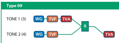
This type passes the filtered sound of each tone through a ring modulator to create new overtones. The tone 1 (3) TVA will control the volume balance of the two tones, adjusting the depth of ring modulator.
