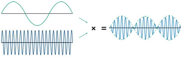
A ring modulator multiplies the waveforms of two tones with each other, generating many new overtones (inharmonic partials) which were not present in either waveform (Unless one of the waveforms is a sine wave, evenly-spaced frequency components will not usually be generated.).
