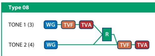
This type sends the filtered tone 1 (3) and tone 2 (4) through a ring modulator, and then mixes in the sound of tone 2 (4) and applies a filter to the result.
