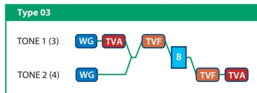
This type mixes the sound of tone 1 (3) and tone 2 (4), applies a filter, and then applies a booster to distort the waveform.
