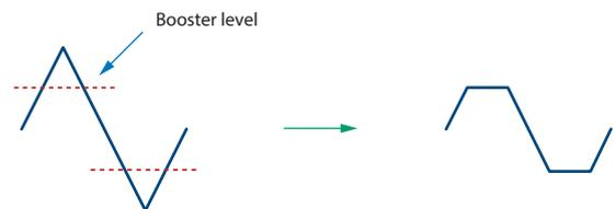
In addition to using this other than to create distortion, you can use the waveform (WG1) of one of the tones as an LFO which shifts the other waveform (WG2) upward or downward to create modulation similar to PWM (pulse width modulation).
