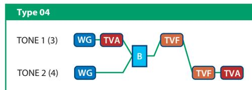
This type applies a booster to distort the waveform, and then combines the two filters. The TVA for tone 1 (or 3) controls the volume balance between the two tones and adjusts booster level.
