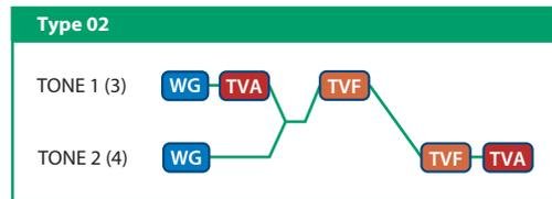
This type stacks the two filters together to intensify the characteristics of the filters. The TVA for tone 1 (or 3) controls the volume balance between the two tones.
